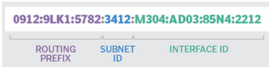
Structure of IPv6 IP-address
