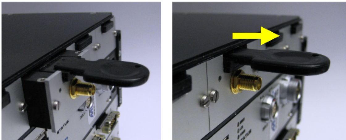
With the tool inserted, the module can be slid out.
