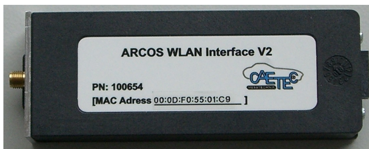
Illus. 2.7.1-2 Bottom view of WLAN module
