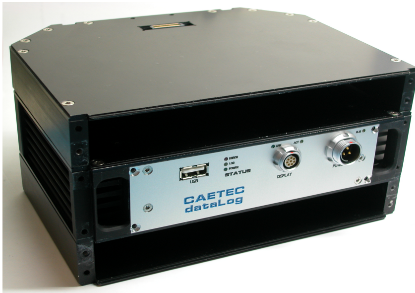
Illus. 2.1-2 The complete logger unit, comprising the basic platform and the chassis units (without slide-in modules)
