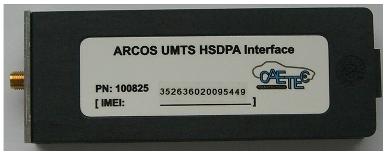
Illus. 2.7.2-2 Bottom view of UMTS module.
